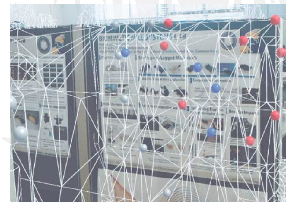
Screenshot of Processed Mesh, showing the red obstacle beacons and blue text beacons
