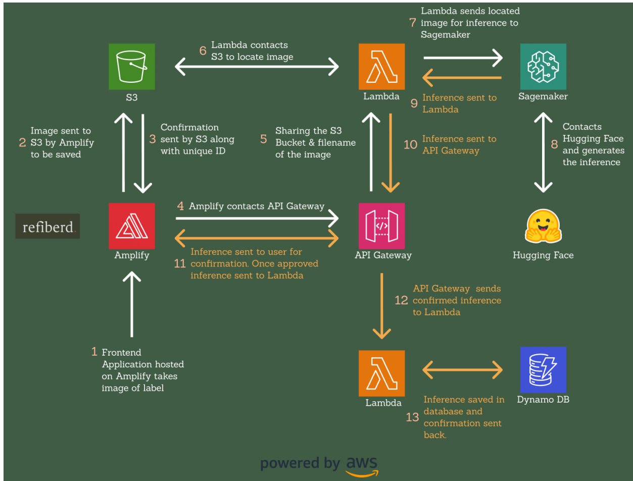
Figure 5 - End-to-End Application Architecture.
