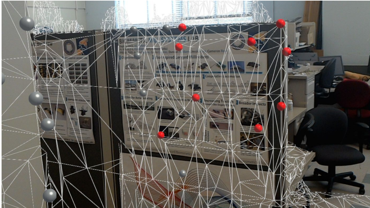
The spatial mesh with obstacle beacons. In Spotlight Mode, only the beacons near the user's gaze would produce sound (as seen here in red).
