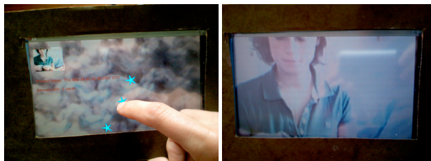
Figure 5 Garment View (left) allowed knitters to access information associated with physical knit by touching points on captured an image of the knit. Touching the image enlarges the captured image (right).
