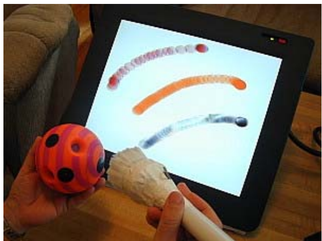
Figure 1. “Picking up” different attributes of an object with the I/O Brush.
